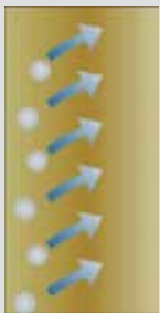
Slowly soluble salts dissolve and migrate towards the surface as the stone dries
