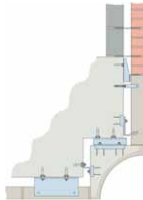
Support unit with special angles and channels for soffit and feature stones
